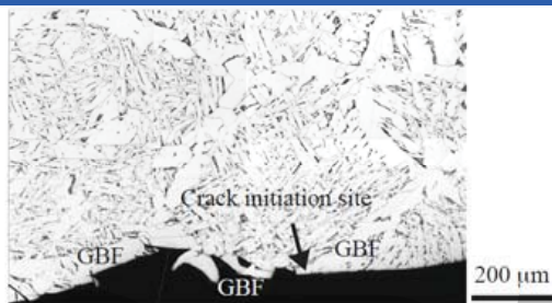
Fig. 1 Microstructure near crack initiation site in HAZ near weld fusion line of electrogas arc welding joint of 490MPa class steel
