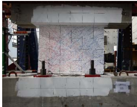
(e) Failure state-front side (3%)
