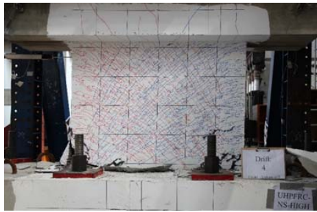
(e) Failure state-front side (4%)
