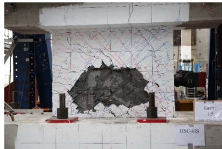
(e) Failure state-front side (1.5%)
