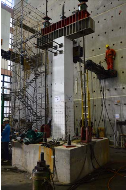
BMRC1 (CIP) B:60cm, f'_c :28MPa SD685:16-D25 SD785:D13@10cm
