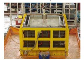
Fig. 1 The instrumented model pile with 6 steel disks on its top in saturated sand specimen on the shaking table
