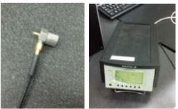
Fig. 9 The higher frequency acceleration gage and data acquisition systems
