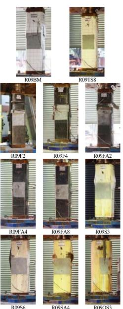
Fig. 8. Failure patterns of specimens
