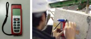
Fig. 8 Infrared gun used to measure distance
