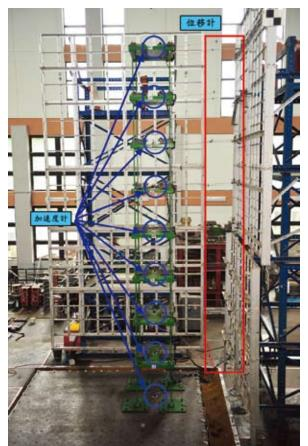
Fig. 1 LVDTs and accelerometers on the eight-story structure
