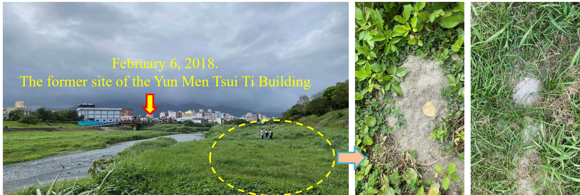
Suspected sand boils possibly caused by soil liquefaction. 73
