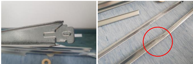
Fig. 38 Ceiling grid and grid connection failure, Zhongxiao Elementary School (PGA: 401 gal).
