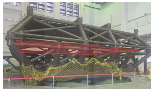
Fig. 3. Test area of the suspended nonstructural system.
