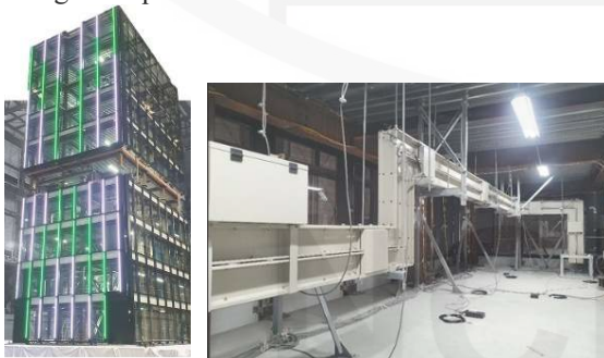
Fig. 1. Ten-story steel frame and 7th-floor busway specimen.
