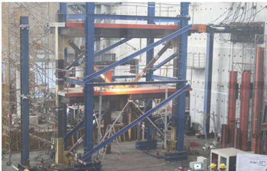
Fig. 7. Full-scale two-story SCBF.
