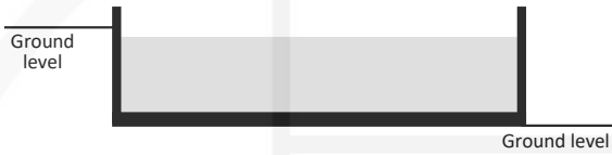
Fig. 3. Side view of a tank positioned on uneven terrain.
