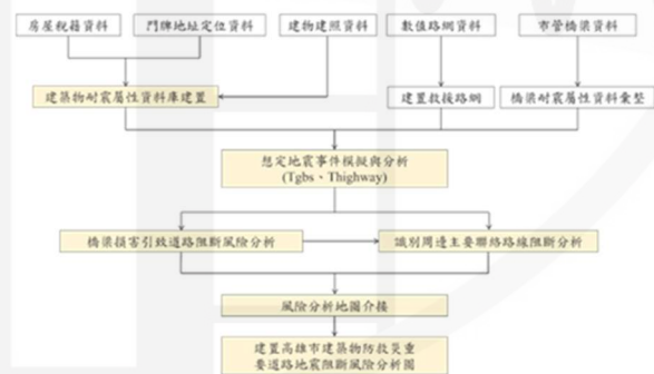
Fig. 5. Workflow of earthquake simulation and road blockage analysis
