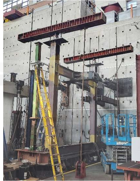
Fig. 5. Full-scale, single-bay MRF.
