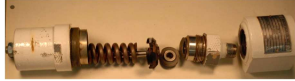
Fig. 3. Failed pressure relief valve component at the Emeryville bus hydrogen refueling station (Harris et al., 2012).
