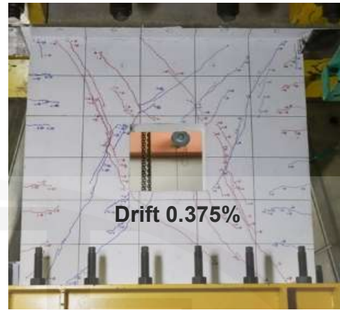
(a) Drift angle reaches 0.375%
