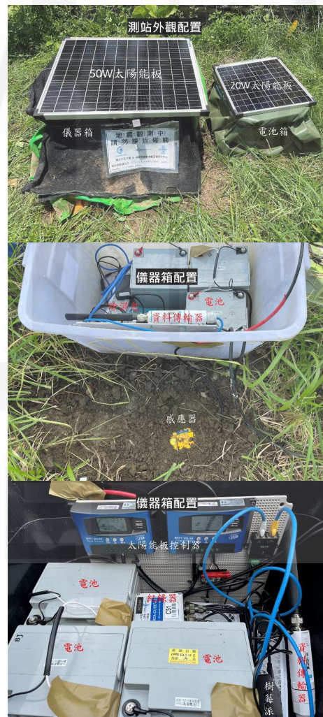
Fig. 3. Configuration of the short-period seismic stations.
