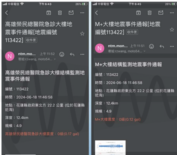
Fig. 3. Notification of earthquake event information for structural monitoring.
