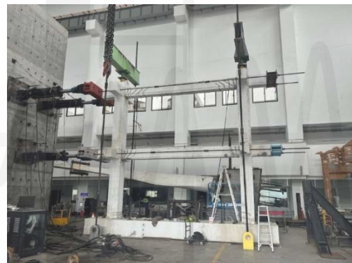
Fig. 6. Test setup of the RC frame
