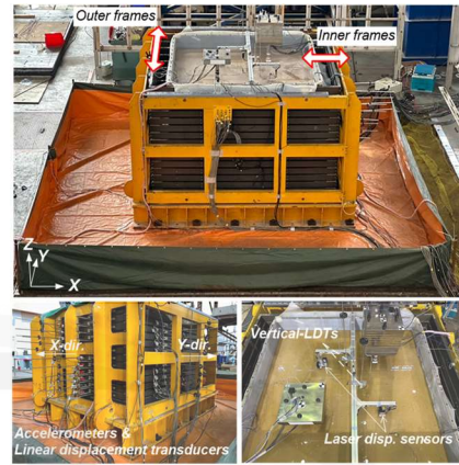
Fig. 2. Actual experimental set-up of the shaking table test
