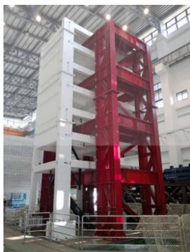
Fig. 1 Seven-story weak-story frame structure
