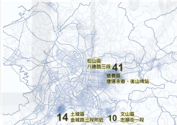
Fig. 3. Gas-related disaster heatmap for the Taipei area during the 0403 earthquake.
