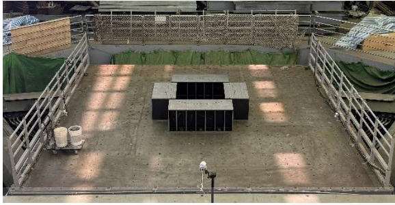
Fig. 6. Jigs secured to the shaking table
