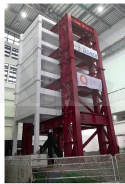
Fig. 2 Torsional behavior of frame structure
