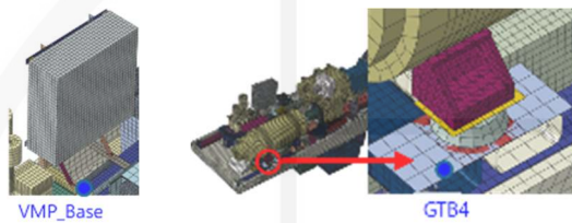
Fig. 13. Output points of VMP controller and generator anchorage points
