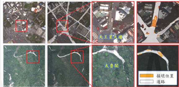
Fig. 7 0403 Hualien earthquake: Image recognition for road damage detection.
