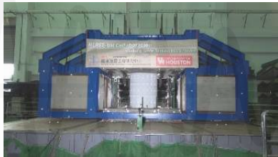
Fig. 5. Test setup with mass blocks for Phase I
