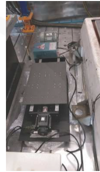
Fig. 5. The small-scale uniaxial long-stroke shaking table.
