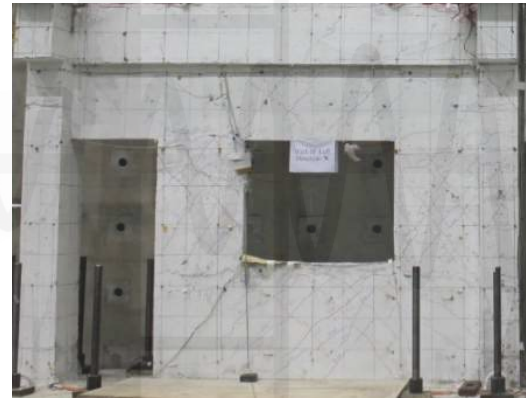
(a) Drift angle reaches 0.37%
