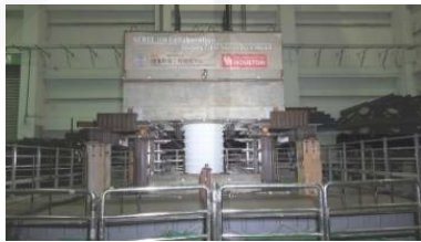
Fig. 4. Test setup with mass blocks for Phase I
