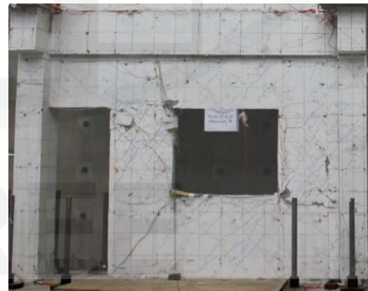
(b) Drift angle reaches 0.62%
