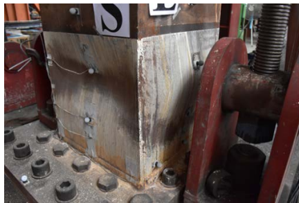
Figure 6 Local buckling at the column bottom observed at 4% drift ratio
