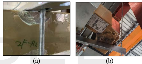
Figure 11. Failure of line elements
