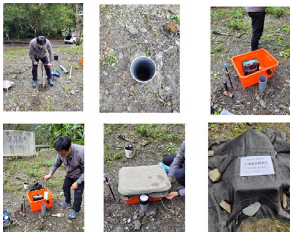
Figure 6. Setting up a temporary radon monitoring station using the RADEX MR107 advanced radon gas detector at Qingshui Geothermal Park.
