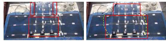
Figure 8. Interfacial debonding failure mode of the PA1 specimen.
