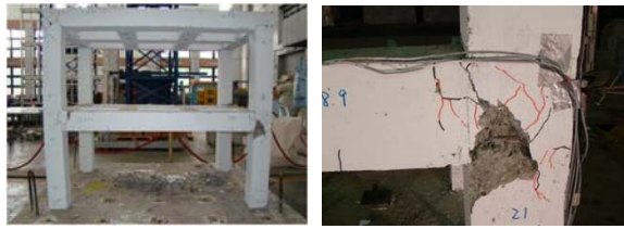
Fig. 5. Failure mode of the frame specimen.
