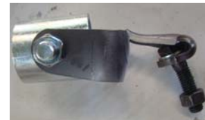
Fig. 5. Failure mode for the shear test.
