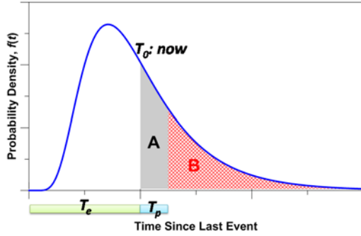
Fig. 2. Diagram illustrating the calculation of conditional probability from a probability density function. The time interval of interest (exposure time) is the gray area (A). The survivor function is equal to the all colored area (A+B). The conditional probability is the ratio of the two areas.
