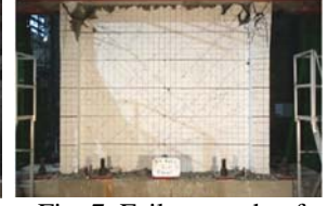
Fig. 7. Failure mode of the specimen SW2
