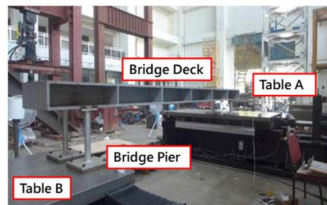
Fig. 4. Experimental setup for multiple tables
